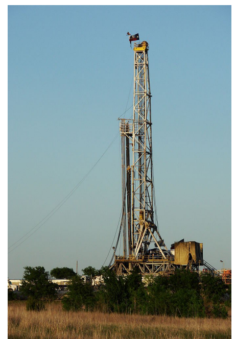
Barnett Shale gas drilling rig, Texas. Photo by David Tribble.
